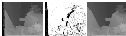
Fig. 7. Disparity map before handling, occlusion candidate, disparity map after handling (from left to right).
