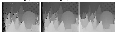
Fig. 8. Disparity maps in each level in a multiscale approach: level 3, 2, 1 (from left to right).
