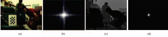
**Fig. 2.** CCD and depth image analysis in the frequency domain: (a) CCD image, (b) FFT result of (a), (c) original depth map, (d) FFT result of (c).
